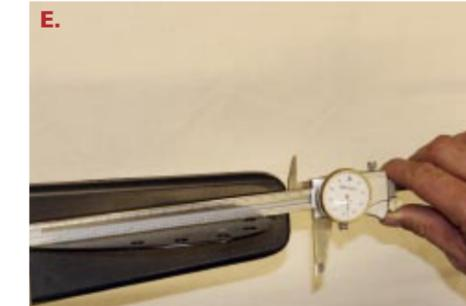
to Tail of Ski Measurement is usually just larger than 8 inches. For users of dial calipers, I recommend that you open your caliper to its 8-inch mark. Then open the caliper to 8.100 and scribe a pencil mark on the caliper. Do this for 8.200 and so on to make taking the Fin Leading Edge to Tail of Ski faster and much less confusing. Users of digital calipers don't need to concern themselves with this.
