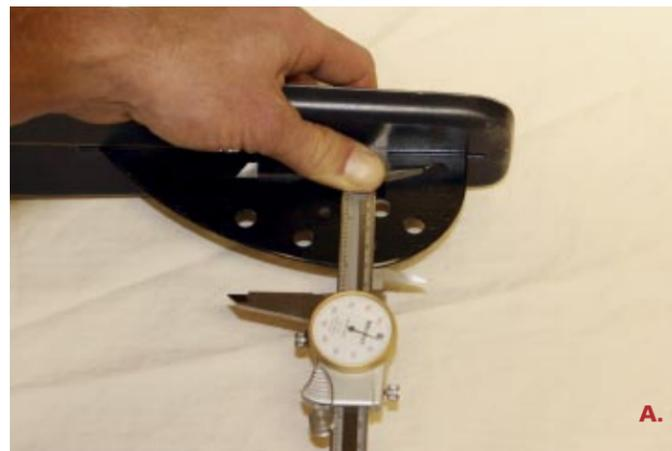
Fin Depth (A) is the point on the fin that is furthest away from the bottom of the ski. Since this is the easiest, most repeatable measurement you can take, I recommend it be your first.
