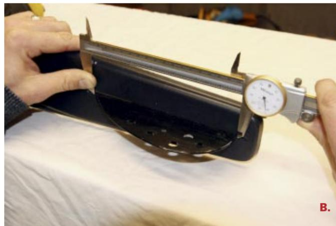
touches the bottom of the ski and the dial extends out past the deepest part of the fin. Hold the nose of the caliper perpendicular to the bottom of the ski with your left thumb and then slide the caliper in with your right hand until it touches the fin. Take a few measurements in slightly different locations.
